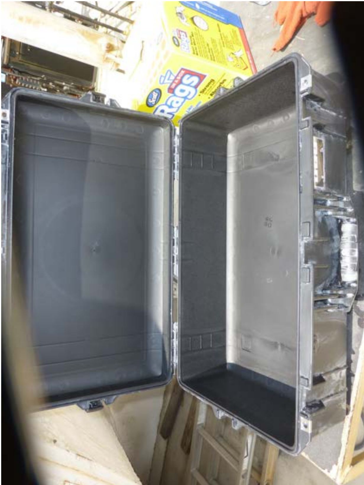
Photograph 15 Immersion - Case 1605 Post Test
