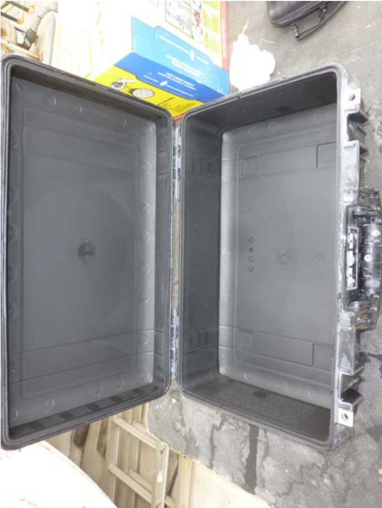
Photograph 6 Immersion - Case 1525 Post Test
