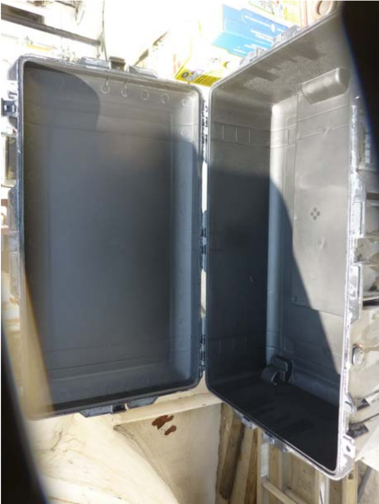
Photograph 18 Immersion - Case 1615 Post Test
