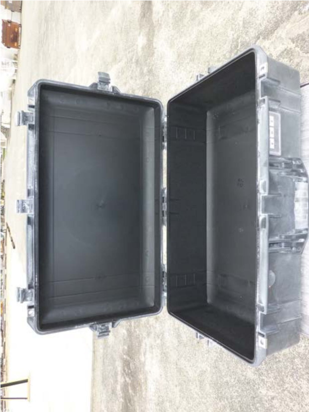
Photograph 21 Dust - Case 1605 Post Test
