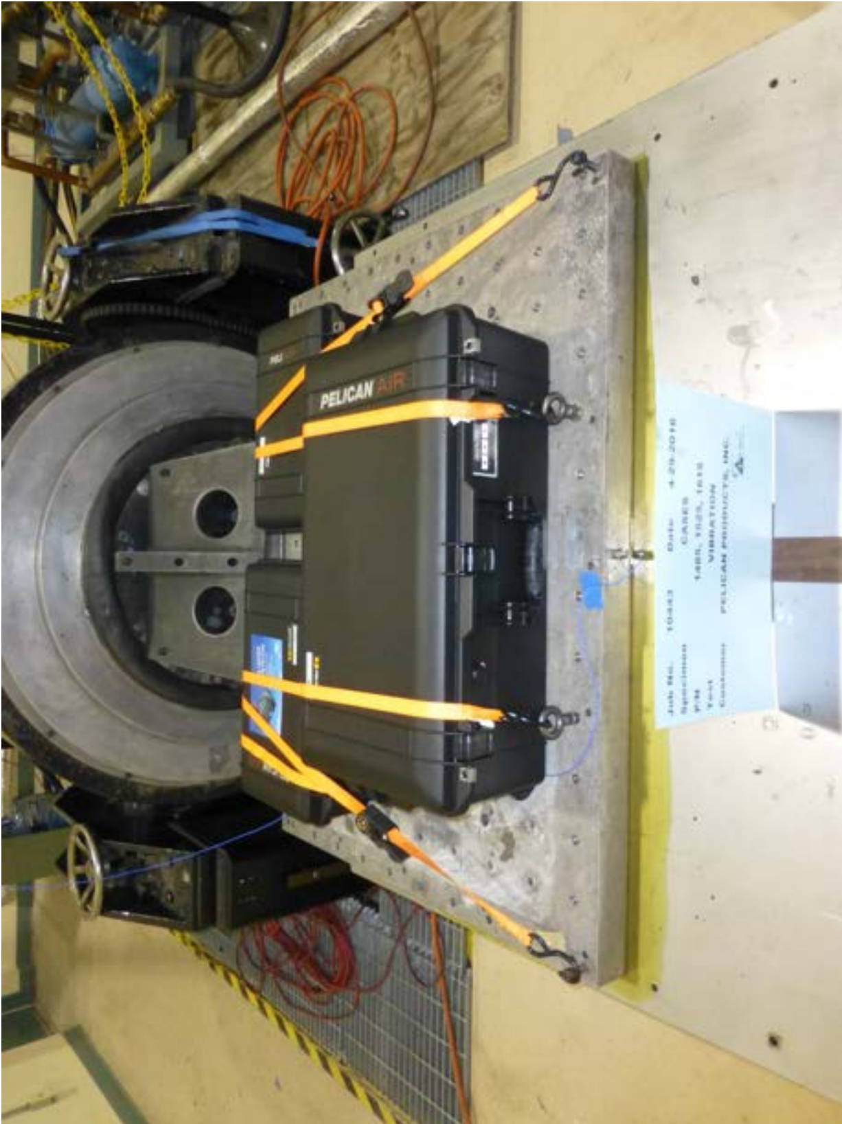
Photograph 3 Vibration - Front to Back - Cases 1485, 1525, 1615
