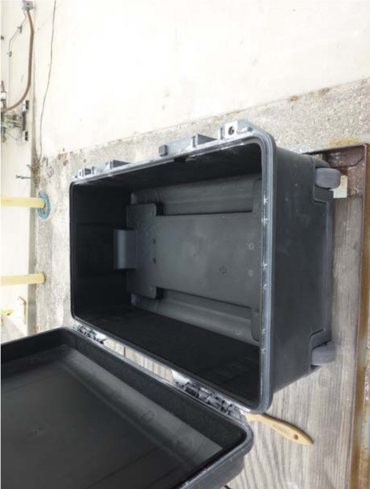
Photograph 7 Dust -Case 1535 Post Test
