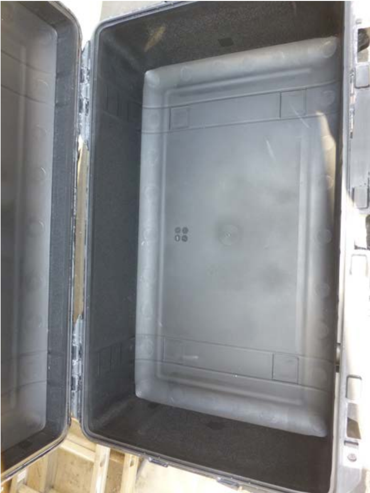
Photograph 12 Immersion - Case 1555 Post Test
