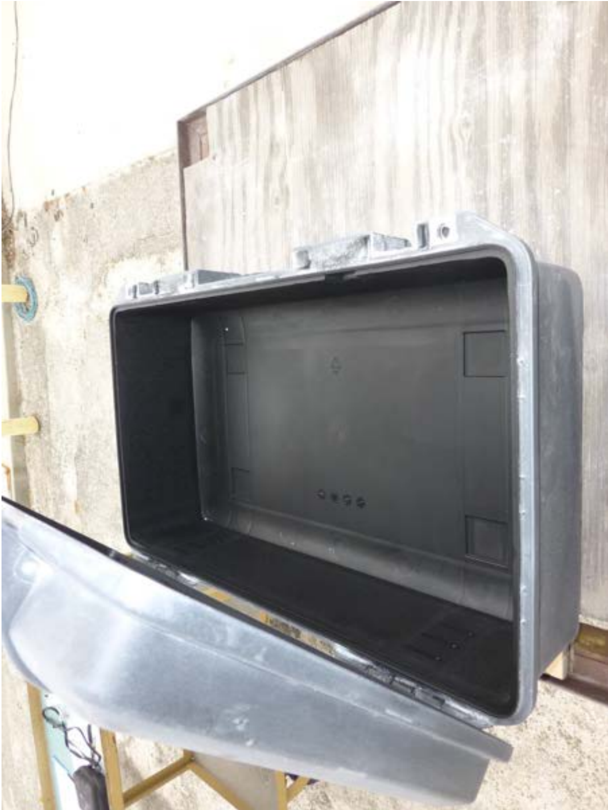
Photograph 10 Dust - Case 1525 Post Test
